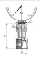
Gauge adaptor, 1/4 BSP to T20 female. Screws direct to T20 test point (M16\*2)
