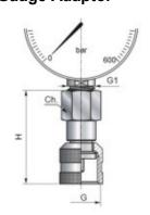
Gauge adaptor, 1/4 BSP to T20 female. Screws direct to T20 test point (M16\*2)
